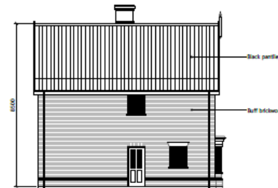
Side (north-west) elevation 1:100
